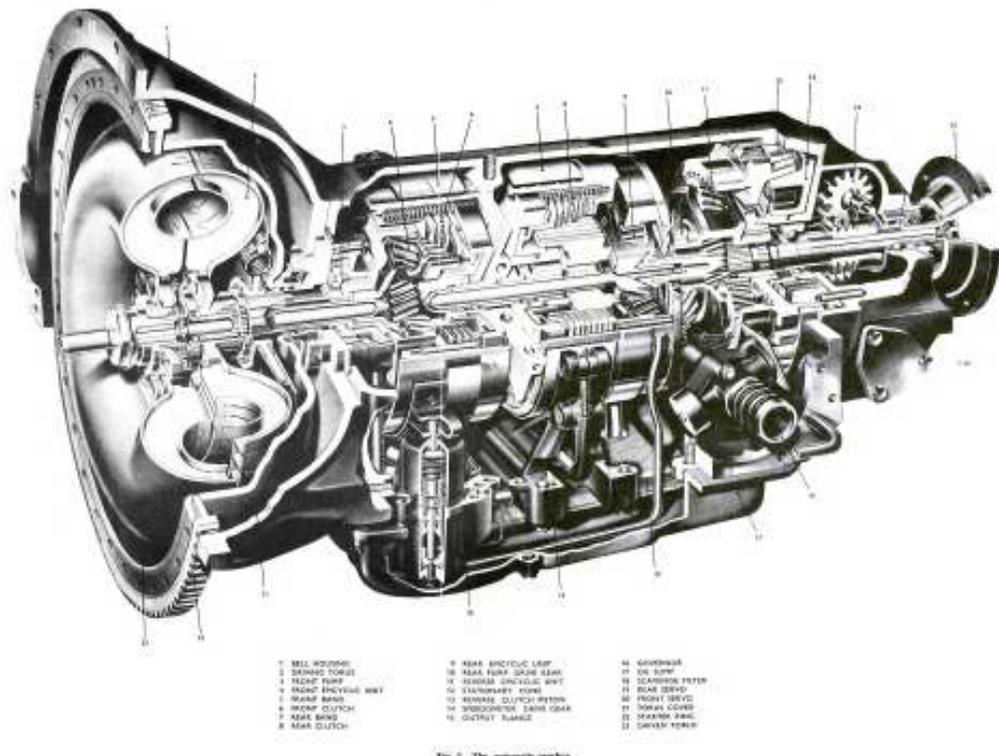
Fig. 2 The automatic gearbox
