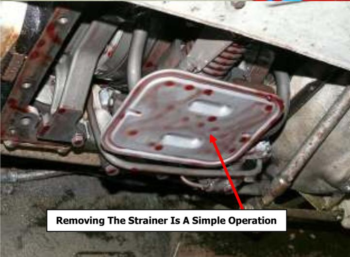
**Removing The Strainer Is A Simple Operation**
