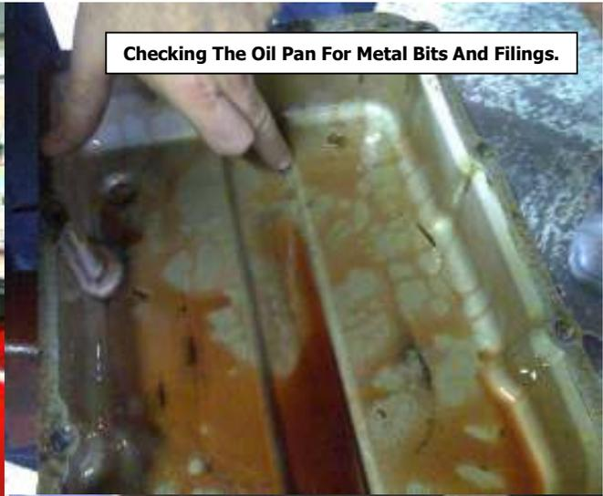
**Checking The Oil Pan For Metal Bits And Filings.**
