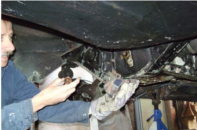
Busy Steve had his hands full this day. Here he changes the diff oil
